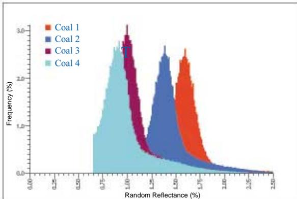
Reflectance Profiles of component coals to be used in making a blend are assembled and the computer mixes them together in the proportions of the desired recipe. This preliminary stage is shown above.
