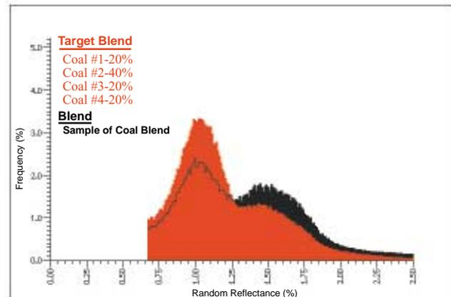
The Reflectance Profile of the computer-built target blend is displayed with the proportions of the components listed. This virtual coal blend can then be compared to a real sample of the blend, as shown above.
