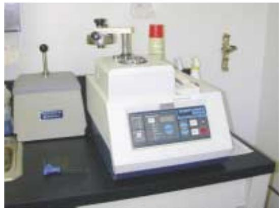
Automated polishing equipment is used to polish six or ten pellets for microscopic examination, in twenty minutes.
